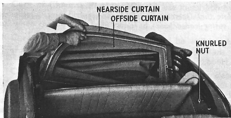
Fig. 25. Placing Curtains in Recess.
